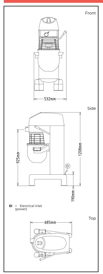
Electric Supply voltage: 200-240 V/1N ph/50/60 Hz **Electrical power max:** 1.01 kW **Total Watts:** 1.01 kW Capacity: Performance (up to): 6 kg/Cycle Capacity: 20 litres Key Information: External dimensions, Width: 532 mm External dimensions, 685 mm Depth: External dimensions,
